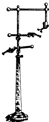
Fig. 17. Valens Multipl Electrode Holder. It is made of mapl and oak and loaded with lead or iron in the base. It can be made by any good wood worker.
