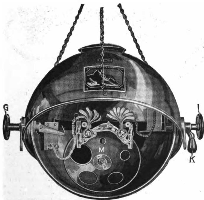
Fig. 180. Heraeus Sun Lamp with reflector lowered to show burner-tilting mecanism and reverse side of selectiv shutter. I is the tilting nob and K is the lock nut for same. G is at one end of the burner holder. M is the selection shutter.
