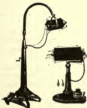
FIG. 32.—Giant and smaller electromagnet. The giant magnet has a lifting power of approximately 400 pounds to the square inch. The smaller electromagnet has a little over one-fourth the strength of the giant magnet.
