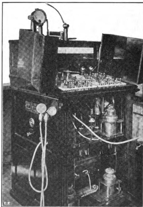
Fig. 26 — Electrical apparatus of extreme compactness, delivering almost all numbers of electrical modalities, including the new "R-rays" (X-ray, High Frequency, Cautery, Ozone, Vibration, Suction, etc.)
