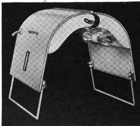
Fig. 49—Local Light and Heat Applicator, shown in Fig. 48 (open).
