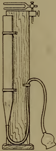
Fig. 64—Showing a Resonance Tube used in my early work in demonstrating the elicitation of the MM VR
