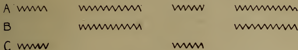
Fig. 88—Shows graphically the modes of current as given thru Valens Metronomic Interrupter when the alternating or rapid-sinusoidal current is passed thru it. Each line represents a cycle of one full respiration.
