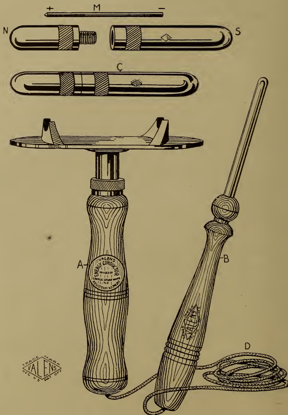
Fig. 2—Pole Differentiating Energy Conductor of 1916. M is a small bar magnet. N and S are the North and South pole respectively. C is an aluminum shell in which the bar magnet is kept. A is the dispersing or subject terminal. B is the receiving or patient-terminal. D is a battery cord.
