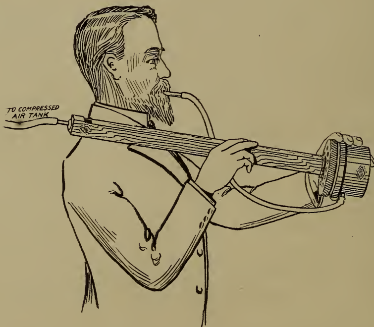
Fig. 43—Changing tension in Practice Drum to change pitch of organ-pipe vibration.
