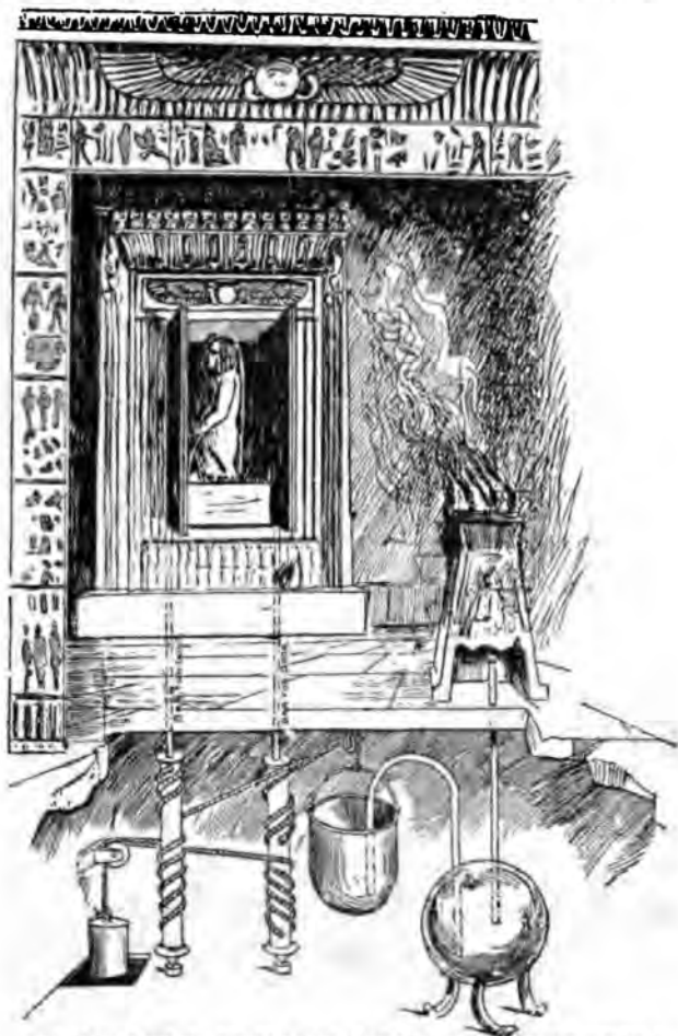
MECHANISM WHICH CAUSED THE TEMPLE DOORS TO OPEN WHEN A FIRE WAS LIGHTED ON THE ALTAR.
