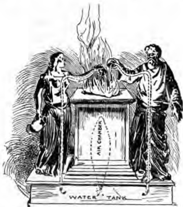
HOW THE STATUES WERE MADE TO POUR LIBATIONS WHEN A FIRE WAS KINDLED ON THE ALTAR.
