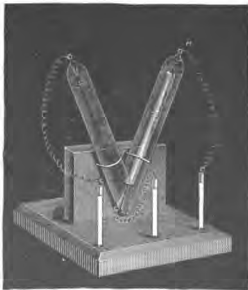
DIAG. 27. — CROOKES'S TUBE. LONG FREE PATH.
