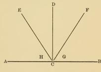
Let A B represent a polished surface, then the perpendicular ray D C falling upon this surface will be thrown directly back from C to D.
