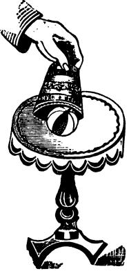
by a mouse, fruit, or any desired article. This cover, the usual height of which is a little over six inches, has within it a scoop, which, in its normal position, presses against the side of the cover, it being thus held by a spring. Connected with the top of the scoop is a brass wire, which goes through the side of the cover, terminating in a little brass button outside. Some are made, however, with the
