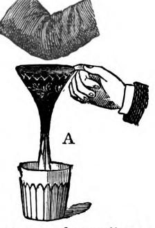
that it has merely the appearance of an ordinary funnel. By placing your finger over the bottom of the funnel at A, and filling it, the inner concealed part also becomes full. There is a small air-vent beneath the handle, and by covering this with the thumb, which can be easily done, and has a most natural appearance when the funnel is held by the handle, all the concealed liquid is kept intact, although that in the funnel proper runs out directly the finger is removed from the bottom.
