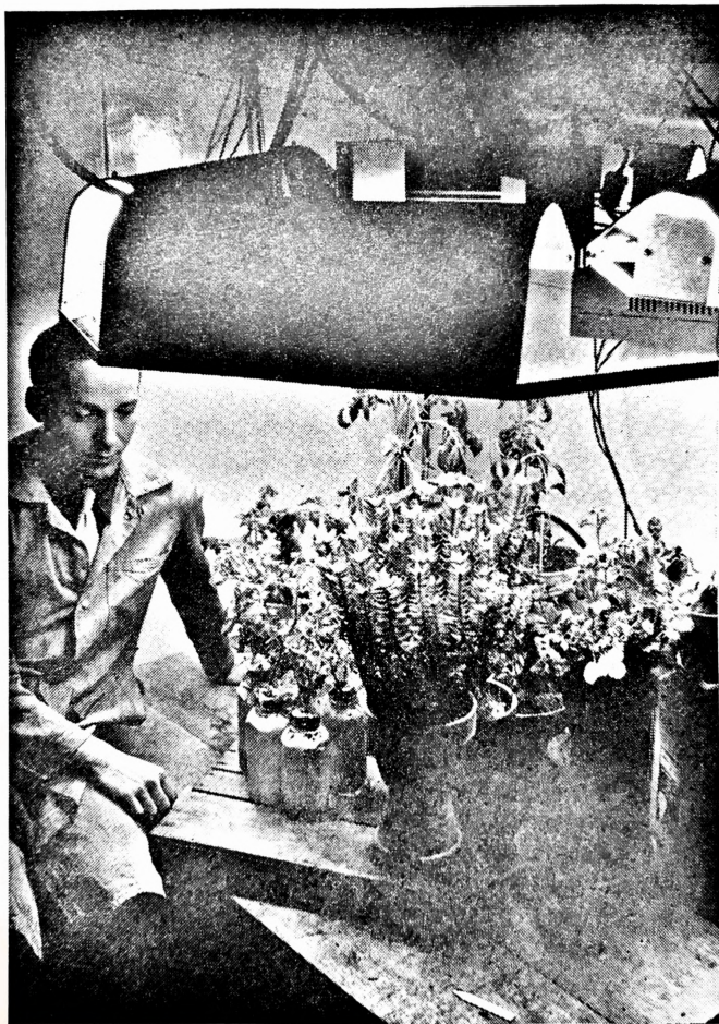
An arrangement of four 10,000 lumen sodium vapor lamps designed especially for plant work
