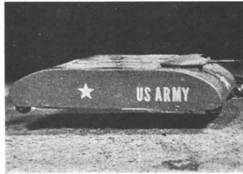
FLYING TANK. Small model shows how a tank can be raised to skim across snow, mud, sand or water.
