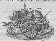
It is more effective than the Steam Fire Engine, be cause it is instantaneously ready and throws a powerful stream of carbonic acid, gas and water for any length of
