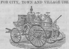
It is more effective than the Steam Fire Engine, because it is instantaneously ready and throws a powerful stream of carbonic acid, gas and water for any length of time.
