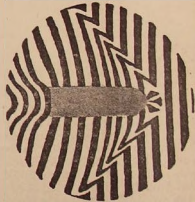
Diagram of a photographed projectile, showing light interference produced by sound-waves it creates in its forward rush. (Copyright by the Open Court Publishing Co.)
