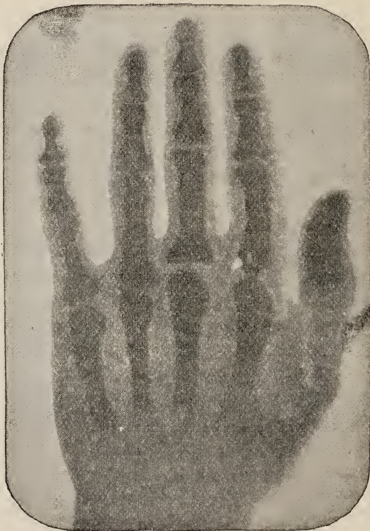
(1) Living Hand through black vulcanised fibre. Exposure four minutes.
