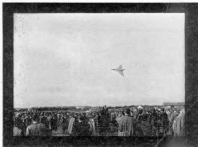
Fig. 1. Photograph of Avro Vulcan aircraft. Ensign Selfix 16-20 camera with 75-mm. Ross Xpres lens. Negative size 2\frac{1}{4} \times 1\frac{1}{8} inches. Length of image on negative 0.42 cm.
