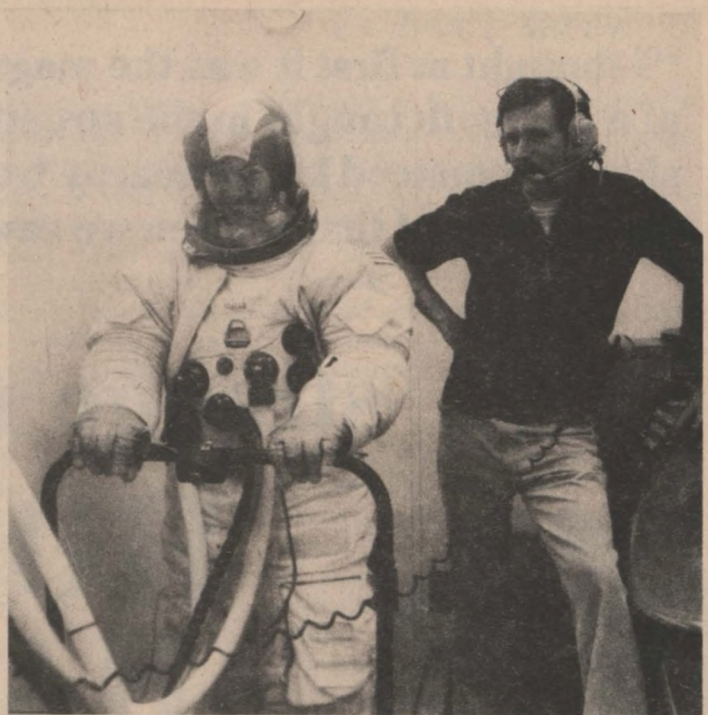
A female test subject wears a liquid cooled garment while exercising on a treadmill in the JSC Environmental Physiology Laboratory. She is Ms. Debbi Guichard of Northrop Service's Inc. Guichard and suit technician Al Rochford (right) are conducting a feasibility study of an automatic comfort controller for Shuttle Mobility Units.
