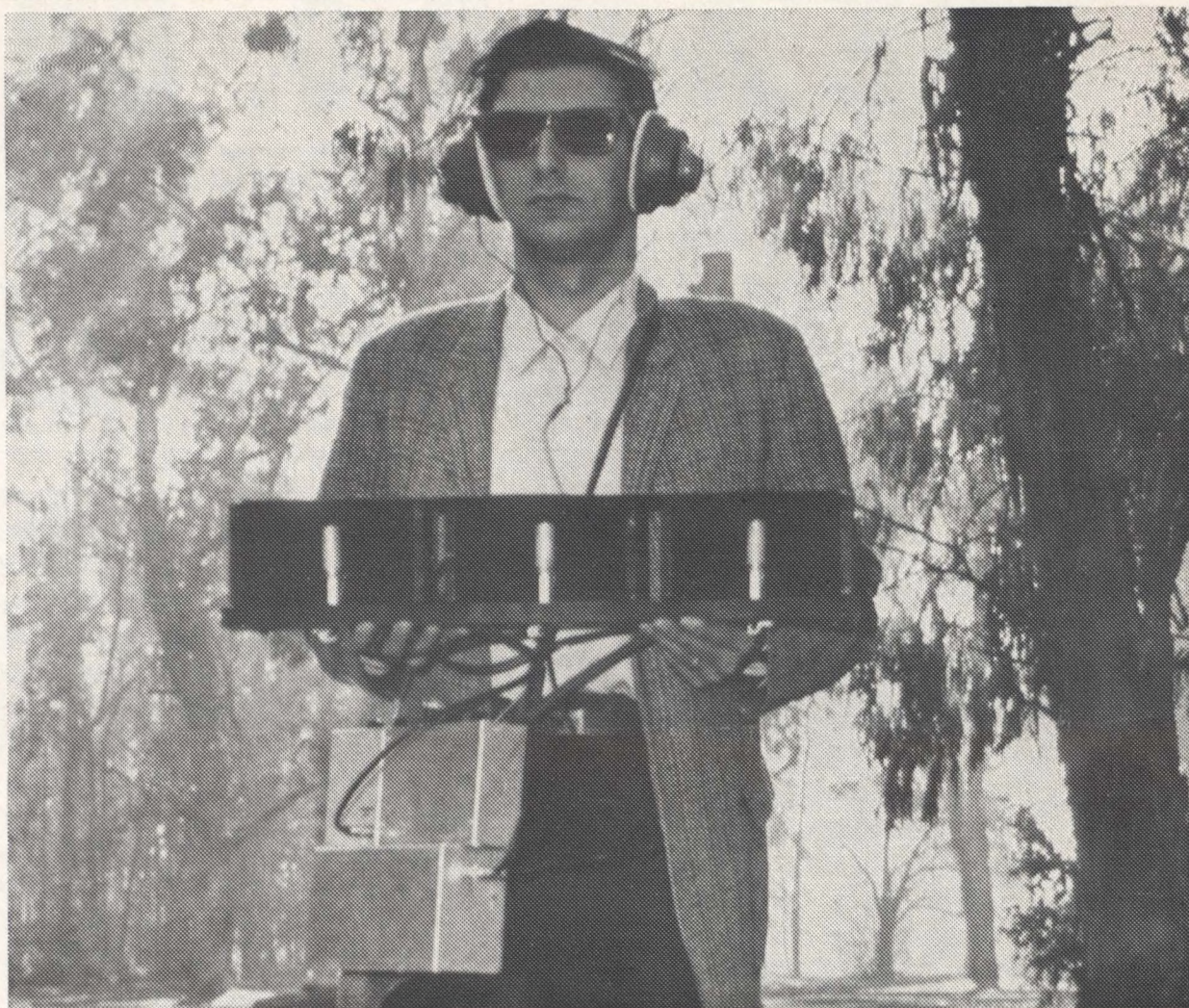
PALO ALTO, Calif., Monday, Sept. 10, 1962—Research scientist Alvin E. Brown, of Lockheed Missile & Space Co., finds his way through a wooded area with a "bat radar" device which uses the principal of the bat hearing system in detecting objects in its path.
